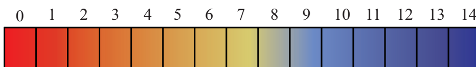
Fig. 8.7: Colour chart/guide of universal indicator/pH paper.
